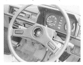
2) Remove steering shaft nut and pull off steering wheel from steering shaft.
