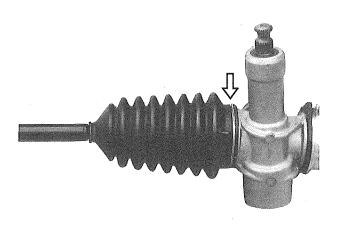
2) Straighten bent lock washer, loosen tie rod ball stud case ① till it is removed from steering rack.
